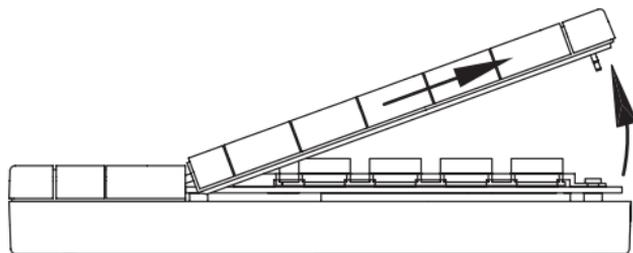
Set the remote control down on the table in front of you with the buttons facing up. Flip the button cover up and pull the cover out of the device at an angle.
