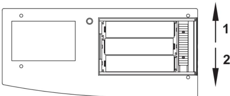
First, open the battery compartment cover as described for changing batteries. A red slider switch is located under the batteries. Push the slider switch in direction 2.
