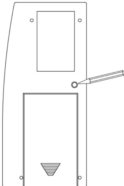
To actuate teach mode on the remote control, press the teach button with a pointed object.
