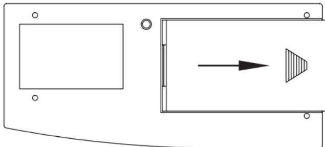
Open the rear battery compartment by pushing the battery cover in the direction of the arrow. Insert the three Micro batteries (Type LR 03) that are supplied and make sure that the polarity matches that of the markings in the battery compartment.
