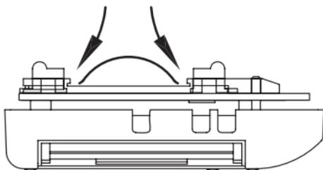
Slip the label card into the slot on one side next to the button to be labeled then. Bow the label card upward slightly to push it through to the opposite side in the slot. The label card should now lay flat on the lighting sheet. Repeat this procedure for all other label cards.
