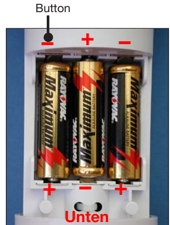
Inserting the batteries; where the button is located
