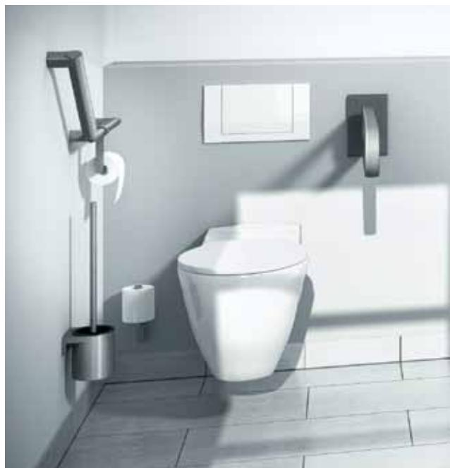
The circulation space of 1500 x 1500mm in front of the WC and the wash basin may overlap, but to the left and the right of the WC there must be a free space of at least 950 x 700mm (width x depth). There must be 300mm spacing from the side of the WC to the wall or fitting.
